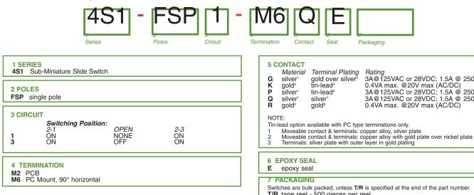
Switches are bulk packed, unless T/R is specified at the end of the part number. T/R tape reel - 500 pieces per reel
